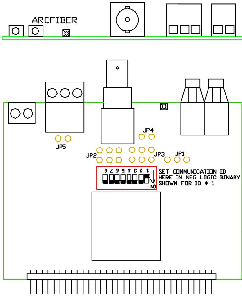
END OF LINE ONLY MUST BVE TERMINATED. USE JUMPER ON CARD OR BNC T AND TERMINATOR
